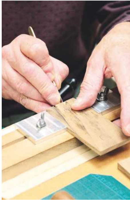
The third jig secures the tail board and allows Robert to transfer the position to the pin board
